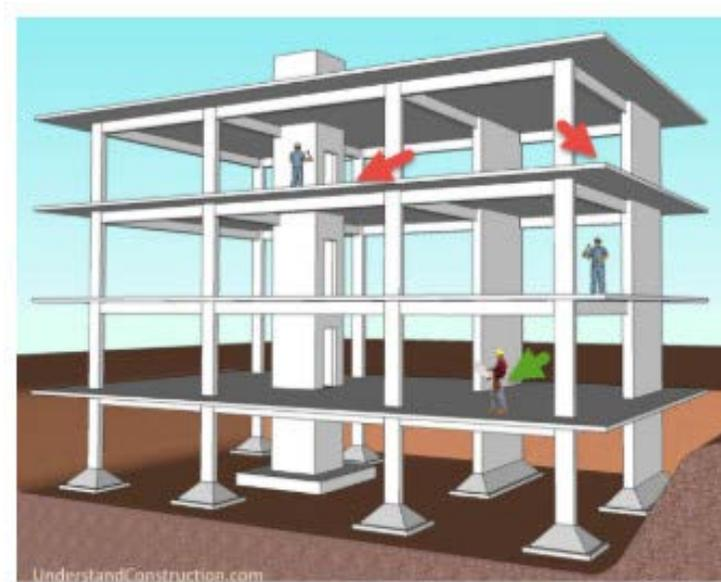
If a building like the schematic above has AC on the roof and an elevator shaft, the two red arrows would not be preferred placements. The green arrow indicates a potential advantageous placement (first floor by a shear wall).
