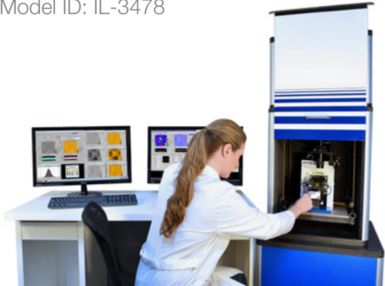
A great advantage of an atomic force microscope is that it can capture several types of images. Each type of image reveals critical information about the surface topography or physical parameters.
